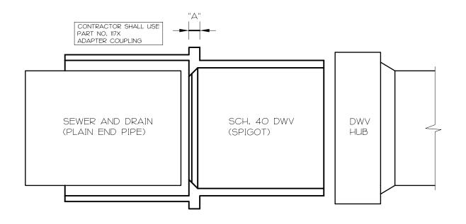
PART NO. 117X ADAPTER COUPLING SEWER AND DRAIN HUB x DWV SPG (ADAPTS SEWER AND DRAIN SPIGOT TO DWV HUB
