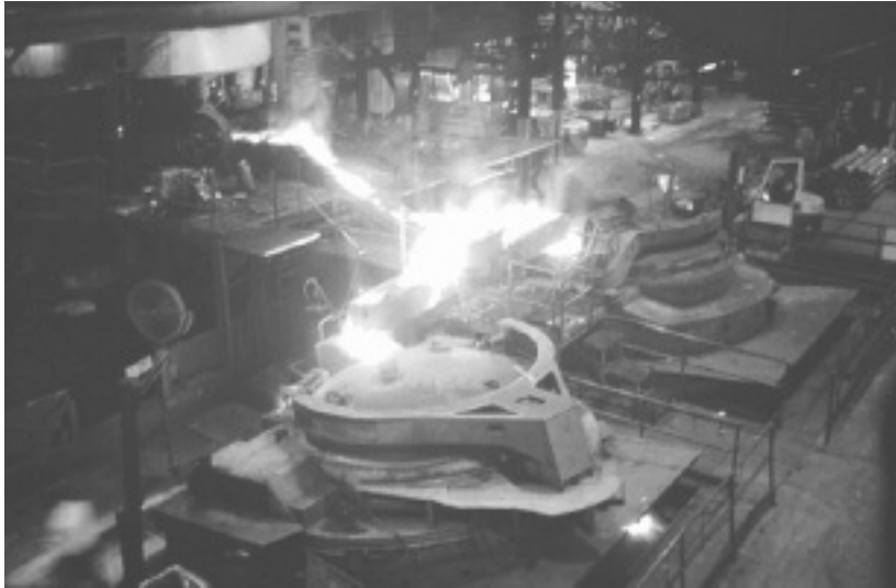
Figure 5—Iron flowing from the Cupola Furnace to Two Holding Ladles.
