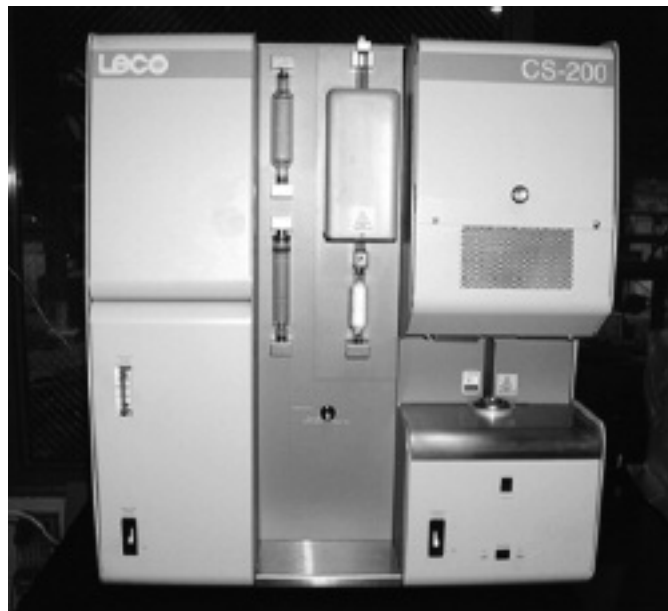
Figure 24—Leco Carbon Sulfur Tester: Used to Determine Carbon Equivalent of Cast Iron. Carbon Equivalent Required by CISPI and ASTM Standards to be 4.10 Minimum by Mass. CE = \%C + \%S_i/3 + \%P/3 .
