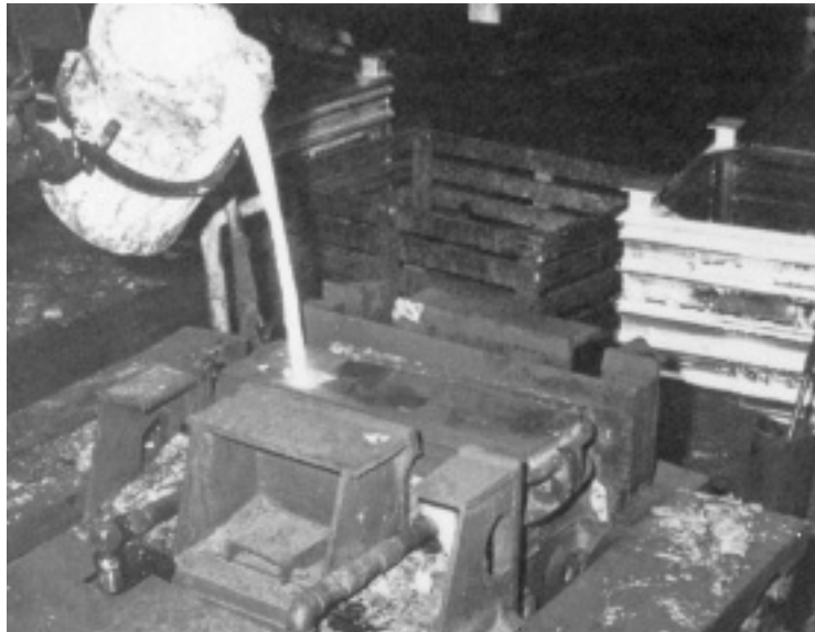
Figure 18—Permanent-Mold Casting for Fittings Production.
