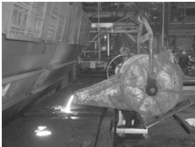
Figure 17—Rotating Wheel-Type Machine for Fittings Production.
