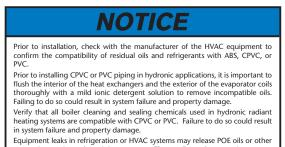
Equipment leaks in refrigeration or HVAC systems may release POE oils or other contaminants into the piping system. These oils and contaminants are incompatible with CPVC or PVC and such exposure may result in pipe or fitting failure regardless of flushing.
